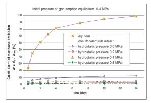
Fig. 7. Comparison of methane emission from the sample of dry coal and coal samples flooded with water at various hydrostatic pressures. Coal taken from No. 361 seam of Pniówek mine
