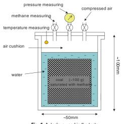
Fig. 5. Autoclave used in the tests
