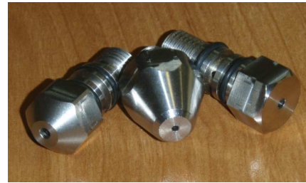
Fig. 2. STK air-and-water spraying nozzles (Prostański 2011b)
