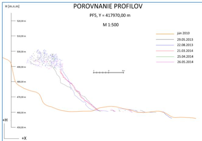
Fig. 10. Comparison of the development of the rock slide quarry walls in profile (graphical scale bar – 20 m)
