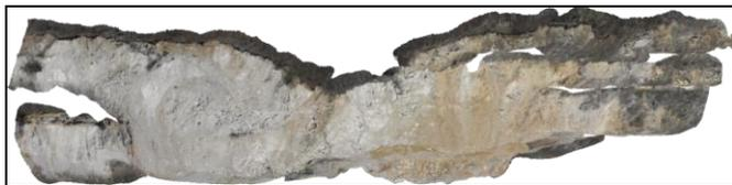
Fig. 8. Orthophotomosaic with a resolution of 0.03 m per pixel, southern view (projection plane XH)
