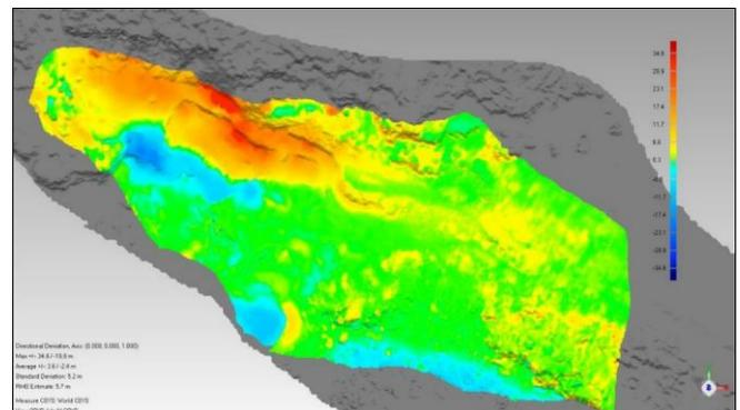
Fig. 9. Surface comparison of TIN models from 2010 and May 2013, top view. Green – no displacements, red – displacements of up to 34 m in the direction of the rock slide, blue – material which has been removed from the quarry
