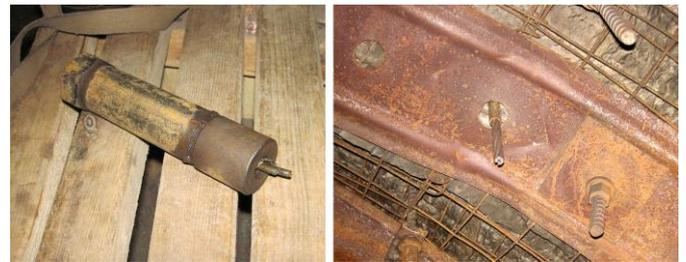
Fig. 14. Breaking away of the locks and bearing plates as a result of an excessive load on the cable bolt
