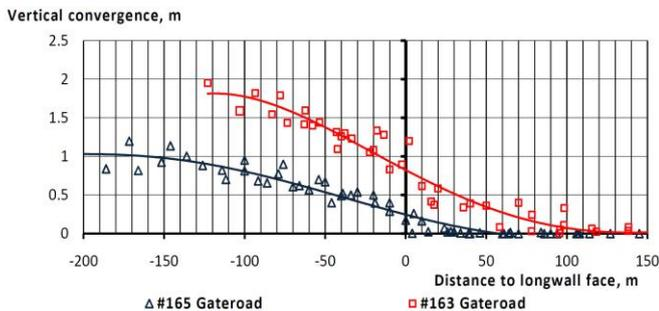
**Fig. 16.** Comparative plot of vertical convergence in gateroads #165 and #163
