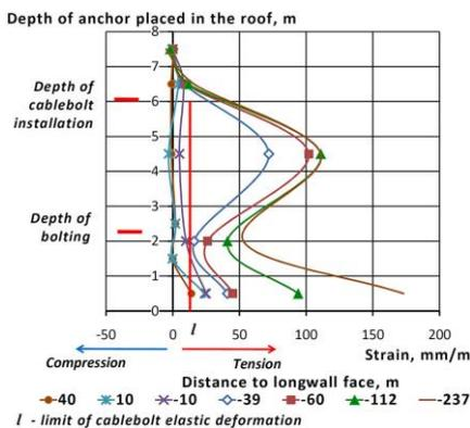
Fig. 13. Vertical strain of rock mass at observation station #3
