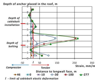
Fig. 9. Vertical strain of rock mass at observation station #1
