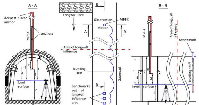
**Fig. 7.** Levelling of "support-rock mass" system elements and anchors of extensometer: 1–5 readings from staff placed on: 1 – top section of steel arch; 2 – gateroad floor; 3 – the deepest placed anchor of the extensometer; 4 – end of steel arch rack; 5 – collar of the borehole of extensometer; 6 – displacements of the anchors of extensometer with respect to the deepest (highest) placed anchor
