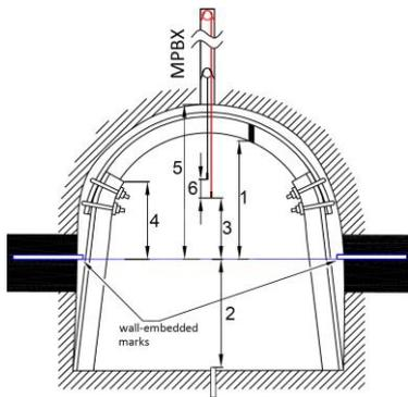
**Fig. 5.** Typical observations of the displacement of support elements and rock mass: 1–5 – linear measurements from the level of wall-embedded marks to: 1 – top section of steel arch; 2 – gateroad floor; 3 – the deepest placed anchor of the extensometer; 4 – end of steel arch rack; 5 – collar of the borehole of extensometer; 6 – displacement of the anchors of extensometer with respect to the deepest (highest) placed anchor
