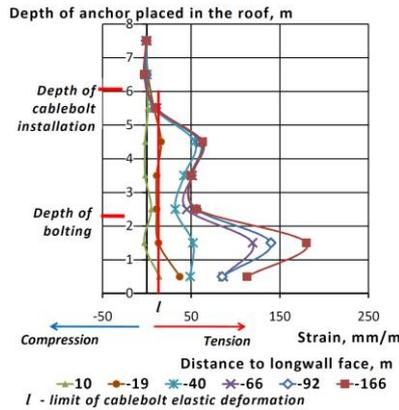
Fig. 11. Vertical strain of rock mass at observation station #2
