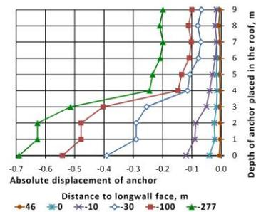
Fig. 8. Absolute displacement of extensometer anchors at observation station #1
