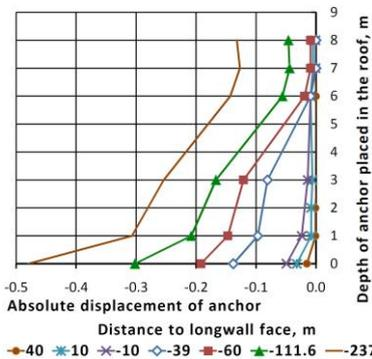
Fig. 12. Absolute displacement of extensometer anchors at observation station #3
