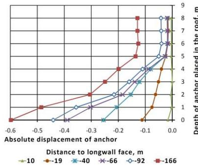
Fig. 10. Absolute displacement of extensometer anchors at observation station #2
