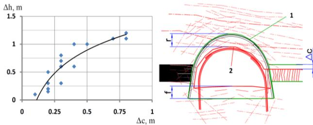
**Fig. 15.** Dependence of vertical convergence in gateroad ( $\Delta h$ ) on the sagging of the roof over the roadside pack at the border "gateroad-goaf" ( $\Delta c$ ): 1 – contour of the gateroad before deformation; 2 – deformed contour of the gateroad behind the longwall face;  $r$  – roof sag;  $f$  – floor heave;  $\Delta h = r + f$
