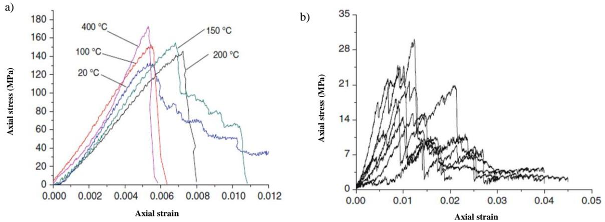
Figure 3. Stress-strain curves of sandstone samples: a – for temperatures in the range of 20–400°C, b – the temperature of 1200°C
