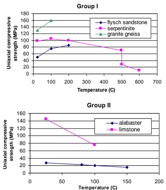
Figure 1. Dependence of uniaxial compressive strength on the temperature: a – crystalline rocks and sedimentary clastic rocks, b – carbonate sedimentary rocks (Pinińska 2007)
