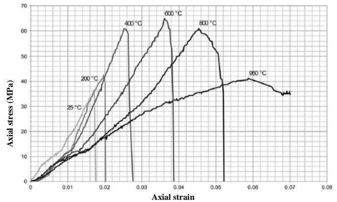
Figure 2. Stress-strain curves of sandstone for temperatures 25–950°C (Ranjith et al. 2012)
