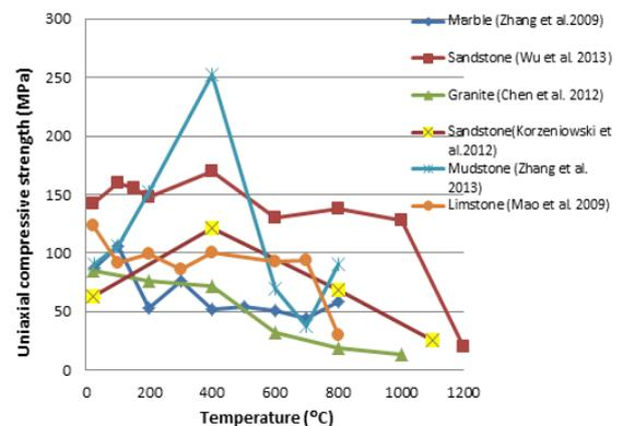
Figure 5. Change of the compressive strength of selected types of rocks subjected to high temperatures
