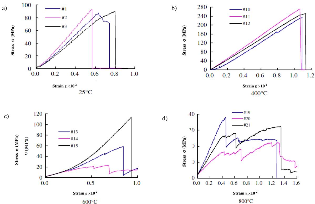
Figure 4. Stress-strain characteristics of mudstones: a – 25°C, b – 400°C, c – 600°C, d – 800°C (Zhang et al. 2013)
