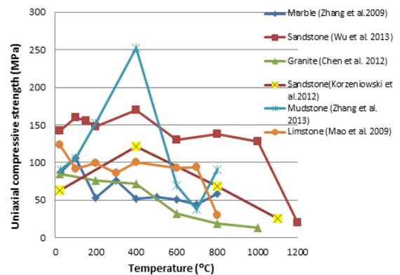
Figure 5. Change of the compressive strength of selected types of rocks subjected to high temperatures
