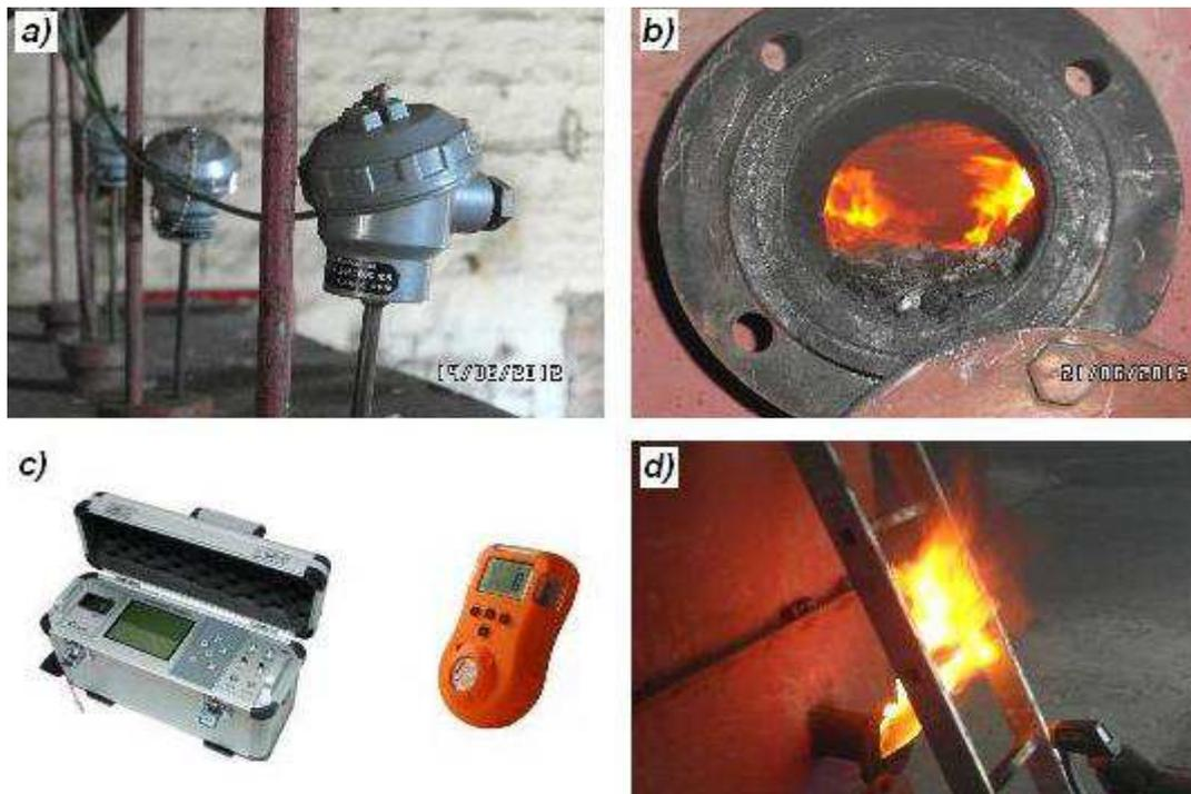
**Figure 2.** Gasification channel ignition with temperature fix: a – thermocouples above combustion face in the stationary mode, b – ignition stage and combustion face burning, c – gas analyzer Gasboard-3200L and BX-170, d – pyrometer in the dynamic mode
