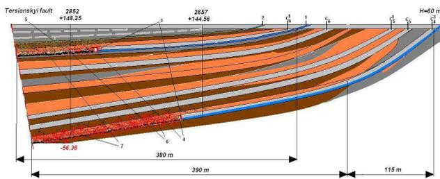
**Figure 6.** Technological scheme of coal seams on area No 1: 1 – inlet borehole, 2 – stowing borehole, 3 – combustion face, 4 – a reaction channel of in situ gasifier, 5 – a stowing rock mass, 6 – goaf, 7 – ash and slag
