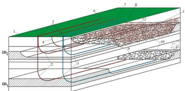
**Figure 7.** Technological scheme of borehole underground coal gasification: 1 – surface, 2 – outlet borehole, 3 – inlet borehole, 4 – stowing borehole, 5 – inlet borehole direction, 6 – direction of gaseous products, 7 – direction of stowing material, 8 – direction of blowing mixture, 9 – gasification channel (30 m), 10 – goaf, 11 – stowing massif, 12 – control retraction point (0.4 m)
