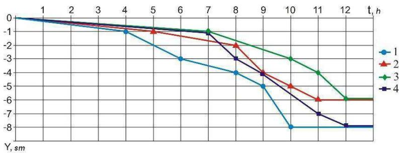
Figure 5. Rocks of roof subsidence in the process of goaf formation
