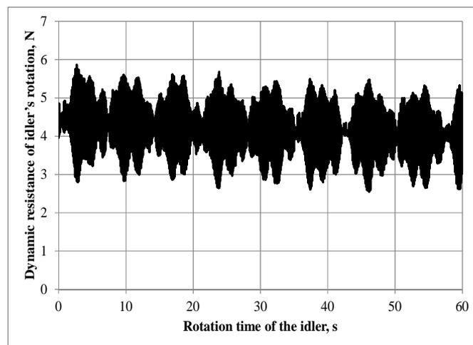
Fig. 10. Test of dynamic resistance of rotation of the idler  $\phi 133$  at a rotational speed of 600 rpm after 4 h of rotation
