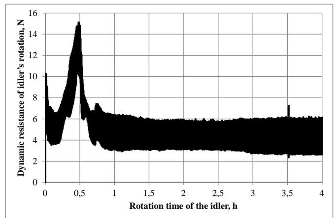
Fig. 16. Test of dynamic resistance of rotation of the idler  $\phi 159$  at a rotational speed of 600 rpm for 4 h
