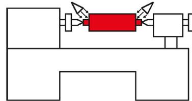
Fig. 5. Diagram of the testing stand which tests the water-tightness of the idler
