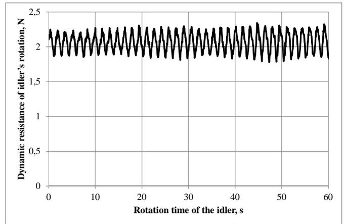
Fig. 14. Test of dynamic resistance of rotation of the idler  $\phi 133$  at a rotational speed of 38 rpm after 4 h of rotation
