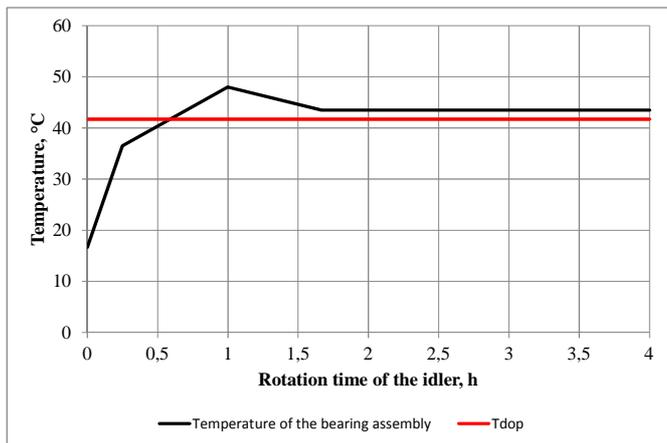
Fig. 17. Test of the temperature of the bearing assembly during the test of dynamic resistance of rotation of the idler  $\phi 159$  at a rotational speed of 600 rpm for 4 h;  $T_{dop}$  – allowable temperature, °C
