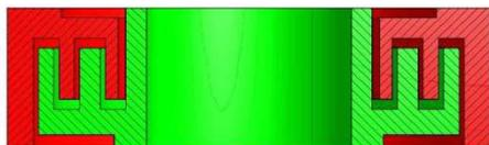
Fig. 2. Typical design of a labyrinth seal
