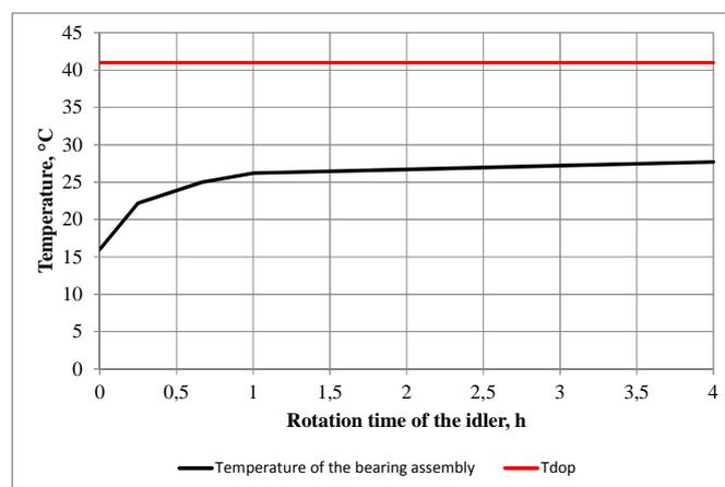
Fig. 9. Test of the temperature of the bearing assembly during the test of dynamic resistance of rotation of the idler  $\phi 133$  at a rotational speed of 600 rpm for 4 h;  $T_{dop}$  – allowable temperature, °C
