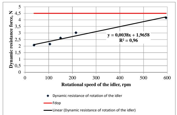
Fig. 15. A graphic chart showing the dependence of dynamic resistance force in the rotational speed function of an idler  $\phi 133$  mm;  $F_{dop}$  – acceptable dynamic rotation resistance
