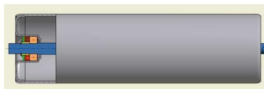
Fig. 3. Bearing assembly with a new seal in accordance with the invention of the Central Mining Institute no. W.121582 (Pytlik, Rabsztyn 2012)
