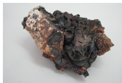
Photo 2. Examples of mineral forms created during thermal transformations of mine waste (Photo by P.Kuna)
